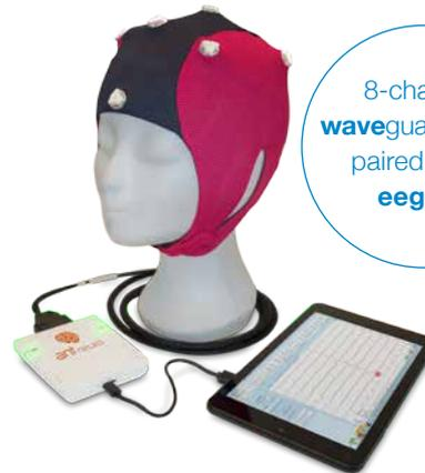
8-channel **waveguard touch** paired to an **eego 8**
